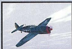
BIG STICK The P-47 packs eight .50-caliber machine guns, making it an excellent mount for ground-attack missions.
